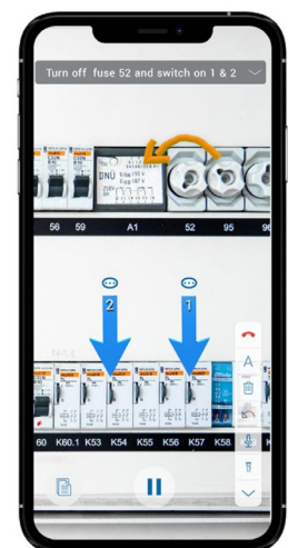
Figure 4: Assist AR support requesters see annotations and visual guides placed on their screen by the remote expert supporter, clarifying every step.
